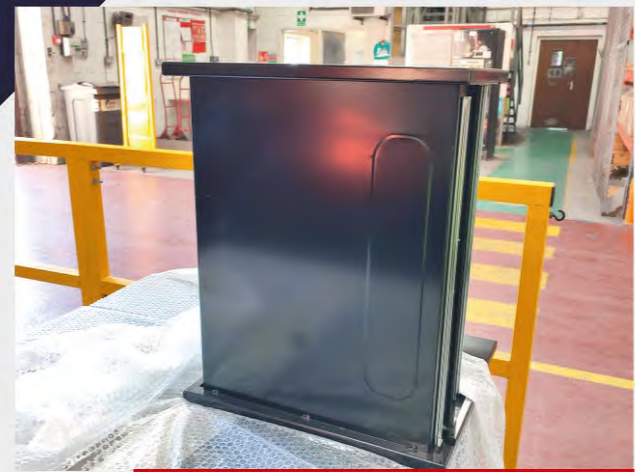
Welded cutout replaced by Punch form
