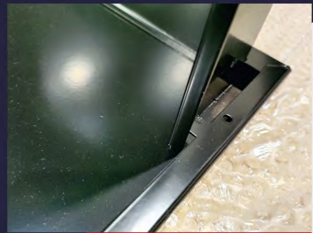
Extended tabs for concealed welds
